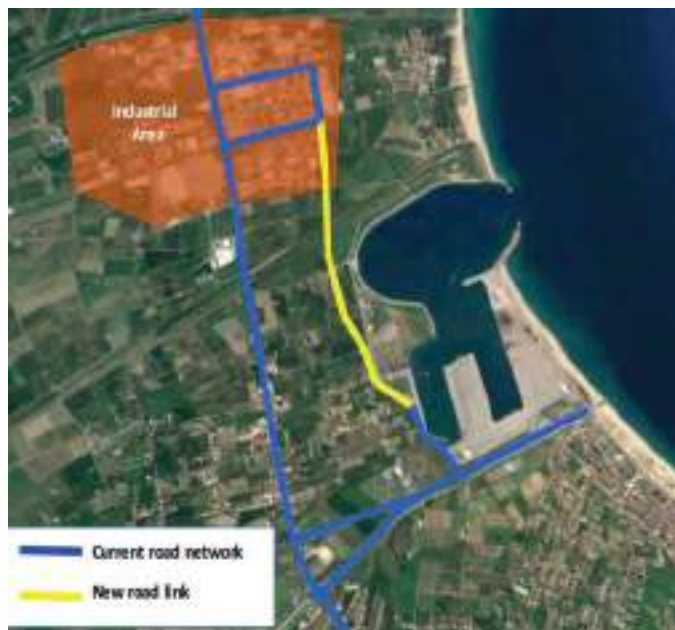
Figure 19 - Road connection between Corigliano port and Industrial Area - Source: UNIMED elaboration
